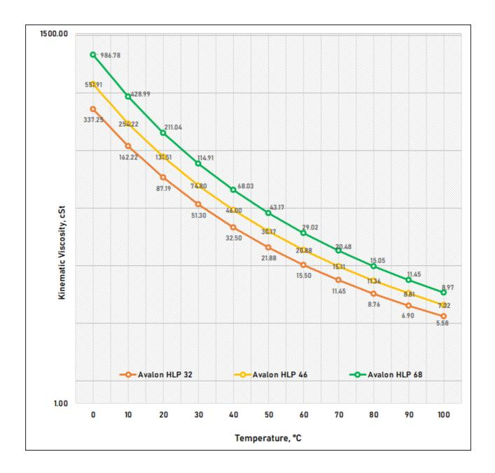
The Viscosity-Temperature Diagram for Avalon HLP is based on the typical characteristics of the product as mentioned above and may vary depending on the batch results having variations that do not affect the product performance.
