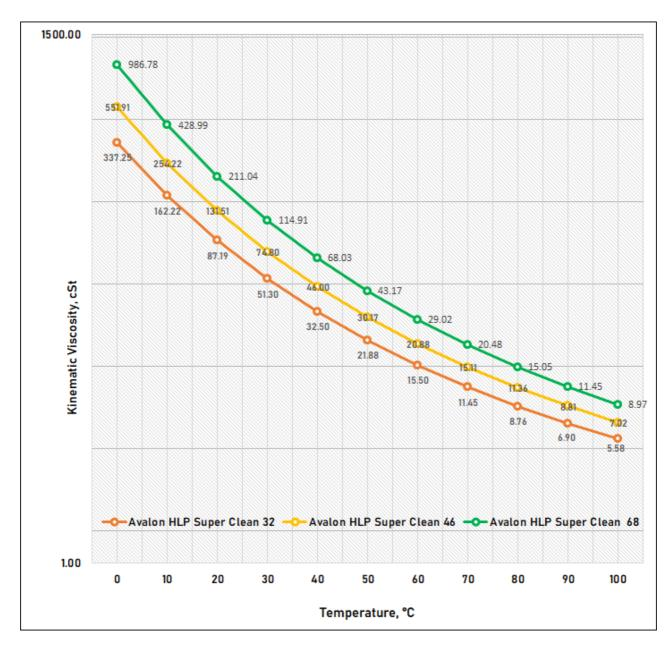
The Viscosity-Temperature Diagram for Avalon HLP Super Clean is based on the typical characteristics as mentioned above and may vary depending on the batch results having variations that do not affect the product performance.
