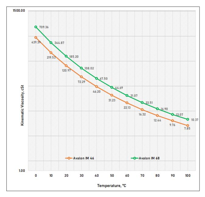
The Viscosity-Temperature Diagram for Avalon IM is based on the typical characteristics as mentioned above and may vary depending on the batch results having variations that do not affect the product performance.
